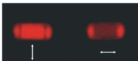
Fig. 7 Polarised fluorescence microscopic pictures of a 2.5 \mu\text{m} long \text{Ox}^+ -loaded zeolite L crystal after excitation at 545–580 nm (cut-off 605 nm). The arrows indicate the transmission direction of the polariser.
